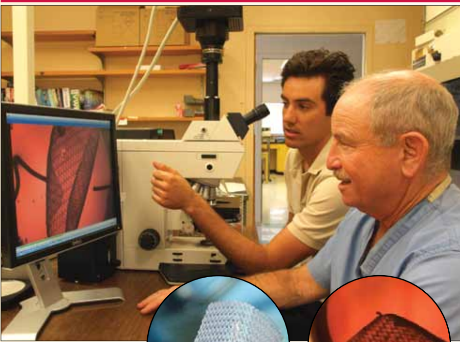
Steven Goldman, MD, (right) and Jordan Lancaster look at an image of the beating patch taken under a microscope. Insets: the patch consists of a mesh of synthetic fibers similar to the material used for surgical sutures (left). When seeded with heart muscle cells and stimulated with electrodes, the mesh begins contracting rhythmically. The cells on the patch are not visible.
