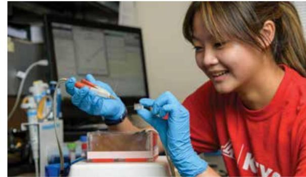
High school student Yi-Jen Yang works on a device that tests whether blood has functioning platelets that can properly aggregate and coagulate.
